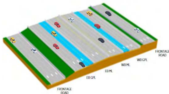
TYPICAL SECTION SEGMENT 1
