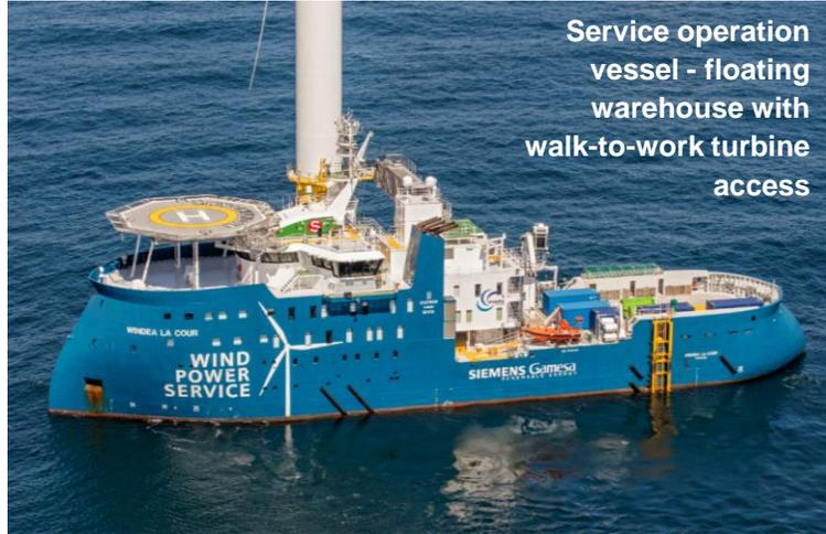
Service operation vessel - floating warehouse with walk-to-work turbine access
