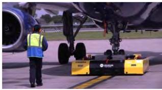
Remote controlled tugs for pushing back aircraft from the jetty
