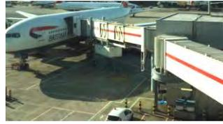
Autonomous jetties speed up boarding and disembarking whilst also reducing accidental damage to aircraft
