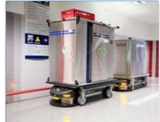
Sacyr currently uses Automated Guided Vehicles for material handling in hospitals under concession. They provide efficient and reliable transport of supplies, linens and waste streams.
